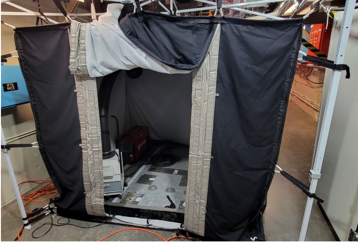
Figure 2 – Faraday Cage for EMI/RFI Protection When Performing Base Mount Welding
